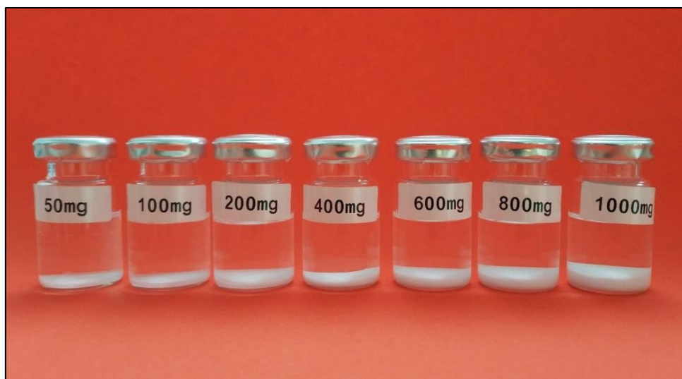
Fig. 3: Sodium tartrate dihydrate in methanol. The salt is sparsely soluble in methanol, making it impossible to visually assess if water extraction has been completed.
