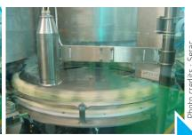
After installation of **ultrasonic defoaming**, the **production rate** of this application has been risen by **50%**.
